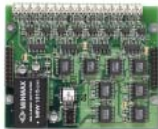
EXP-8V extra 8 voltage output channels
